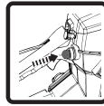
Press primer (4) x6 until the bubble is filled with fuel (cold engine)
