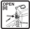
Press the choke lever (5) in, and the throttle is still at fast tickover
